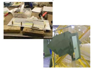
Once we were finished making parts we were asked to make stencils and mark the parts and mark the fuselage as to where they were to be mounted.
