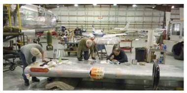
Removed the engines, props and sent them out for over haul and removed all the gear for inspection and repair as necessary.
