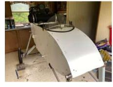
installed (Thanks Ray Robinson), the fuselage has been skinned and has been moved to the garage for center section rigging. As soon as the engine has sufficiently proven itself and the rigging complete, then the outer wing sections will be rigged to the fuselage in the recently prepped hangar at the
