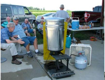
The corn steamer is made from two garbage cans, one inside the other and powered by a propane burner. Worked pretty well, just took longer than originally predicted.
