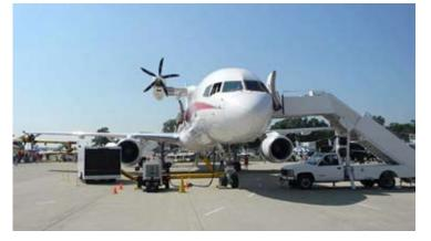
a new special test aircraft with an extra engine;
