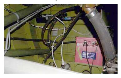
Next was connecting it to a solenoid inside a junction box in the accessary section. From the pic below you can see it was a busy area to work in. The cable is one of the big white ones in the picture. Tidied up some other wires and the project was done.
