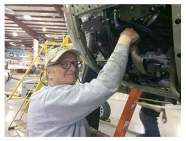
So back out for two engine runs. It turned out the no fuel flow problem was they had not opened the emergency fuel shut off valve for the starboard engine. First to turn the props through. I helped on the port engine and used my shoulder. Not a good idea, I still have a bruise.
