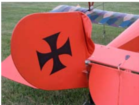
Marvin's Rudder after the Voisin aileron grabbed it.
