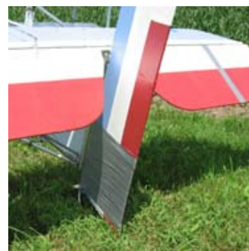
TLAR (above) - Repaired Rudder made it home (below)
